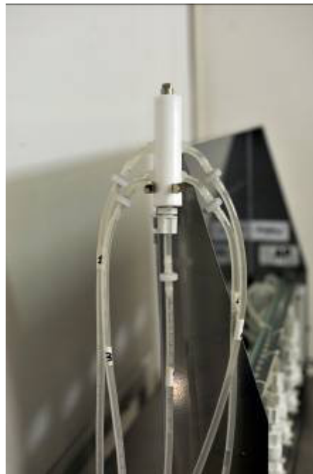
Figure 3: Teflon mouth piece with misting nozzle.
