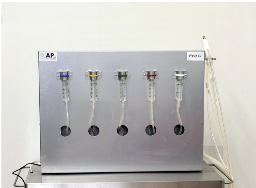
Figure 1: Front panel with flavorant and water vessels. Use Channel #5 (white collar) for fresh water
