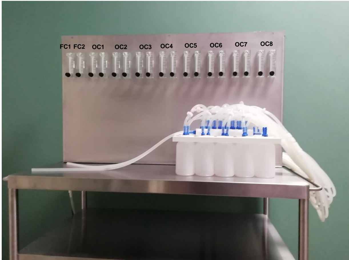
Figure 1: Front panel with flow meters and channel numbers.
