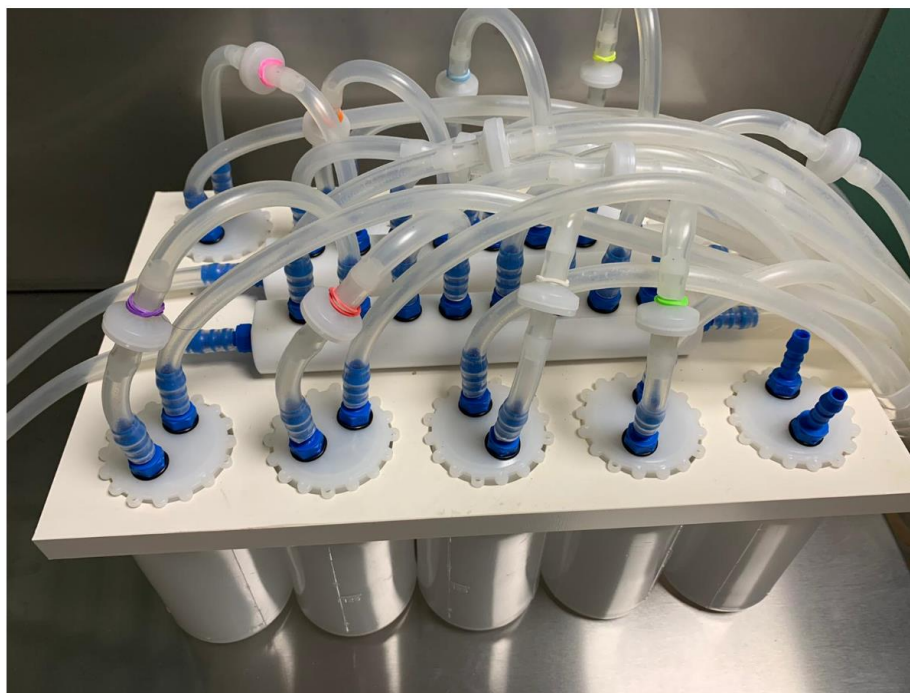
Figure 4: Odorant vial holder with valved connections and outlet manifolds. Odorant subchannels are marked by a coloured ring
