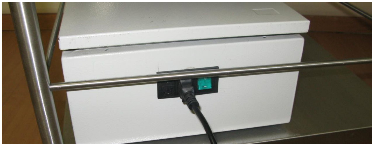
Figure 6: power cable and switch
