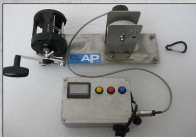
Figure 1. The encoder used in the test
